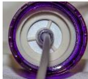
Figure 2: 0.2micron filter inside cap
